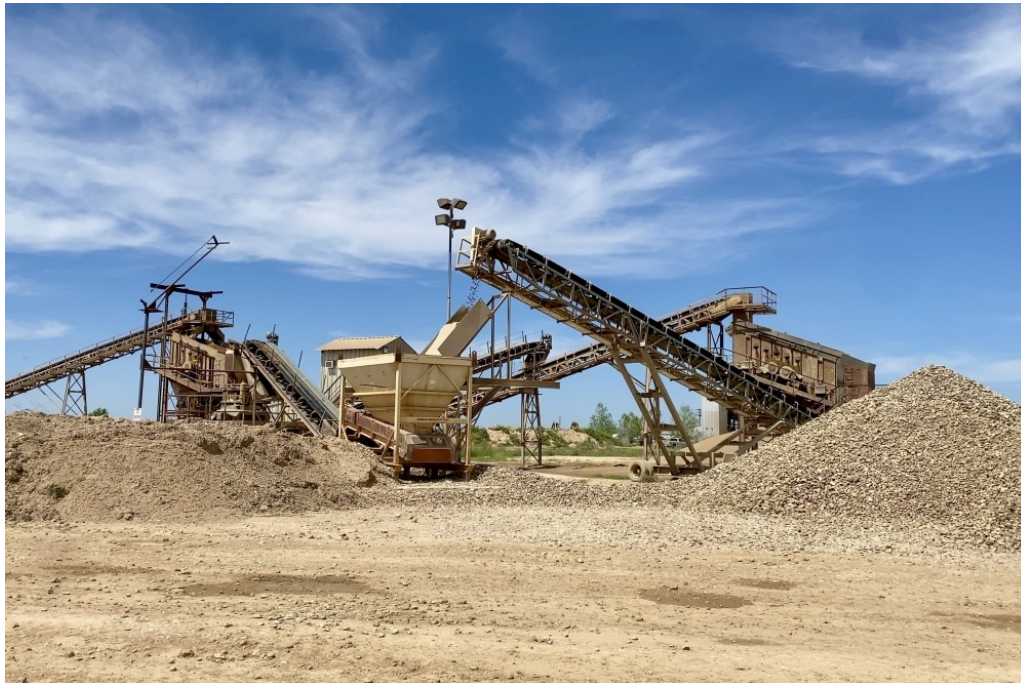
Raw material is then screened, washed and dried. Rock crushing and sorting machines used in this step are often the source of noise concerns. (Jane Turchi/Community Impact)
