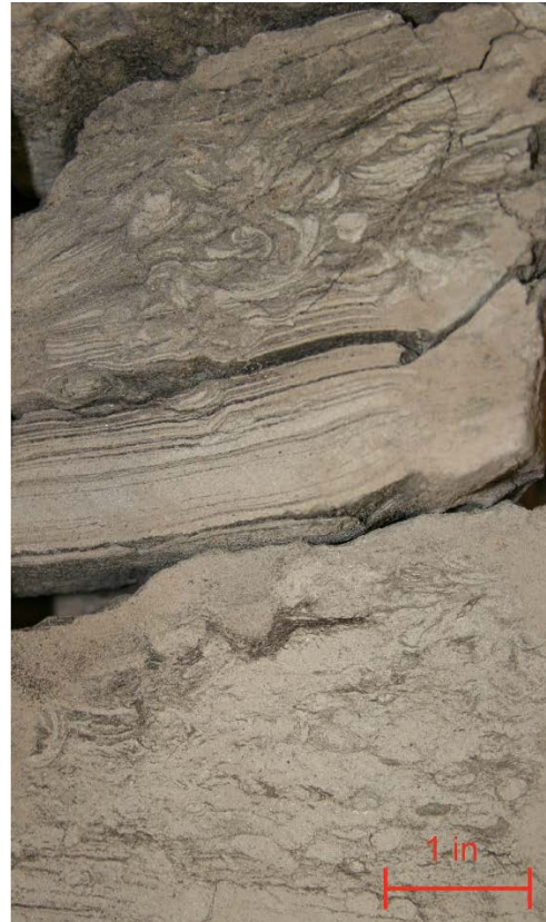
Figure 2.4.2d. Photograph of heavily bioturbated and laminated sandstone, 12923 ft, OCS-G-3496 A-3
