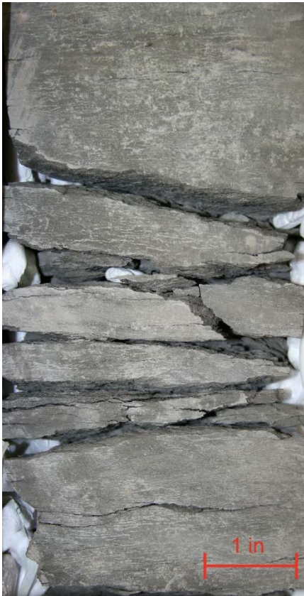
Figure 2.4.2a. Photograph of shaly mudstone, 12963 ft, OCS-G-3496 A-3
