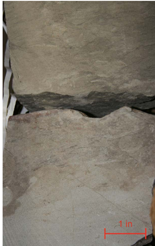
Figure 2.4.2b. Photograph of burrowed mudstone interbedded with sandstone mudstone, 13049 ft, OCS-G-3496 A-3
