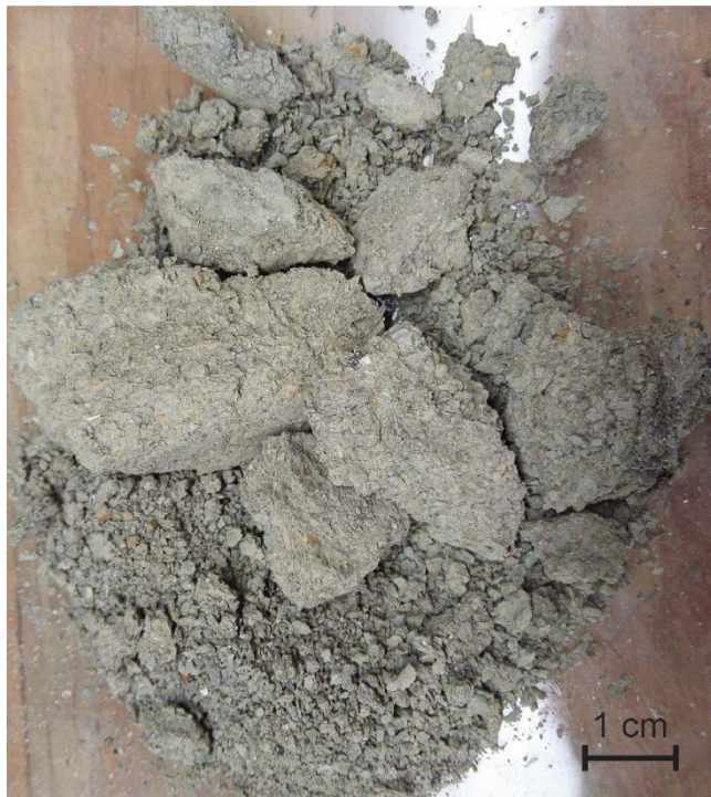
Figure 2.4.13 – Cuttings from OCS-G-4435 #1 contain small, fragile shale flakes not suitable for ion milling and SEM study.
