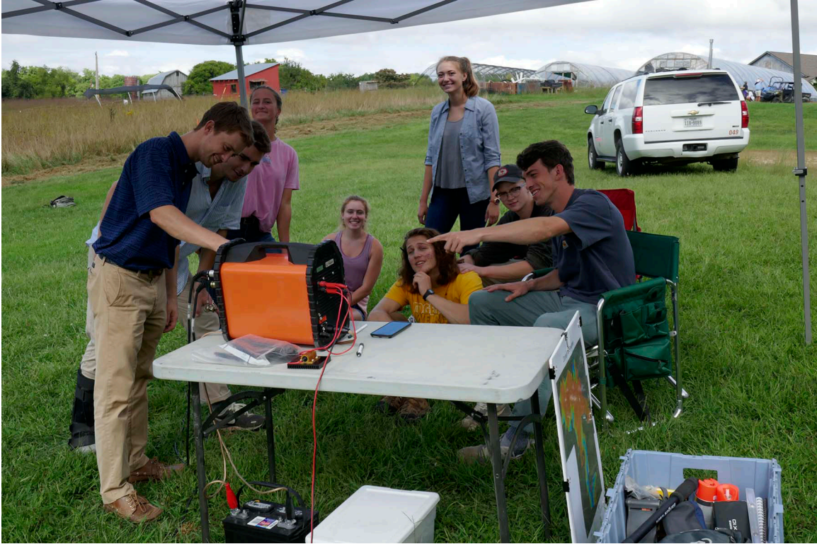
Figure 3. Sewanee students acquiring TDEM sounding data at the Sewanee Farm using a WalkTEM, September 11, 2018.
