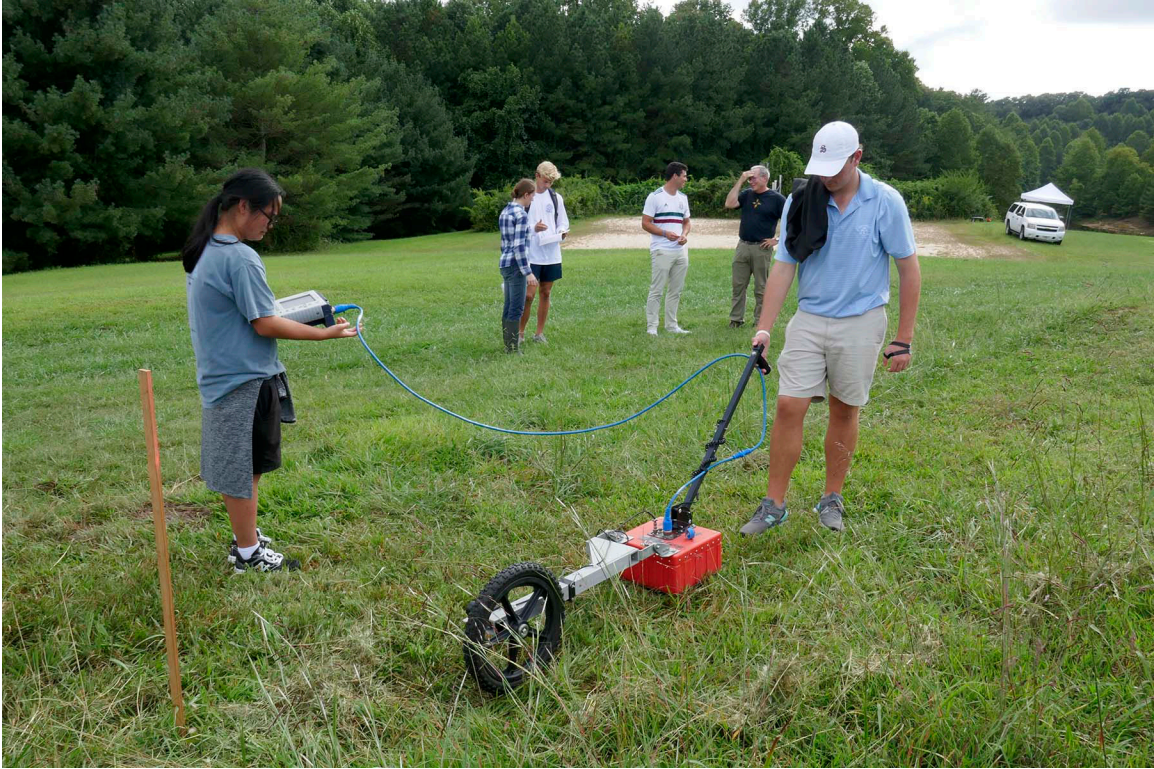
Figure 2. Sewanee students operating GPR instrument along a proposed fence line at the Sewanee Farm, September 11, 2018.
