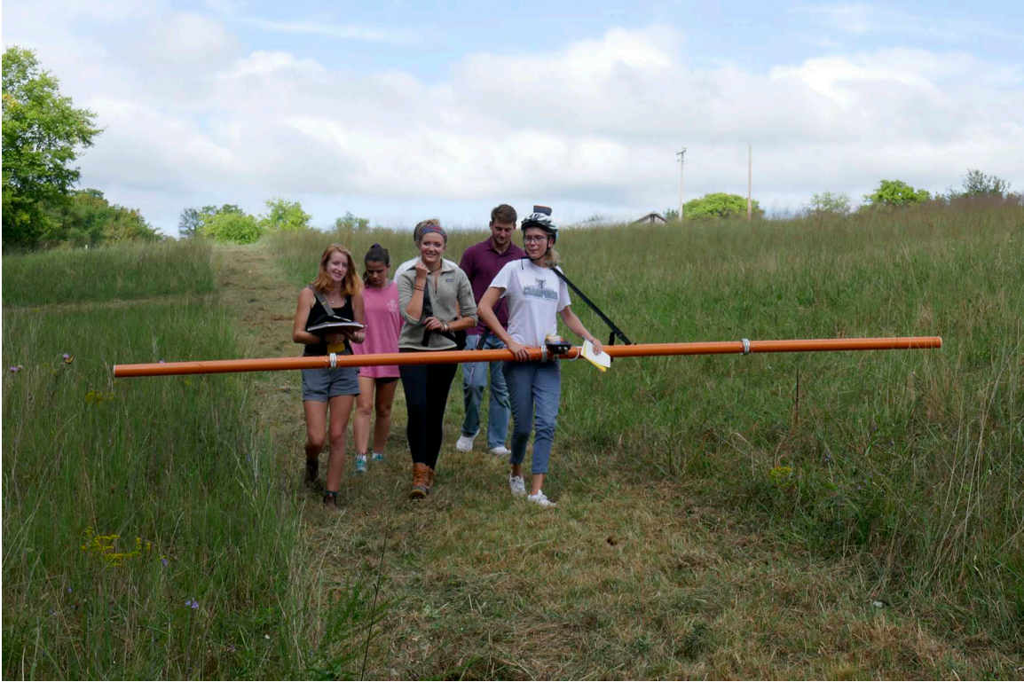
Figure 4. Sewanee students acquiring FDEM data at the Sewanee Farm using the CMD Explorer ground conductivity meter, September 11, 2018.
