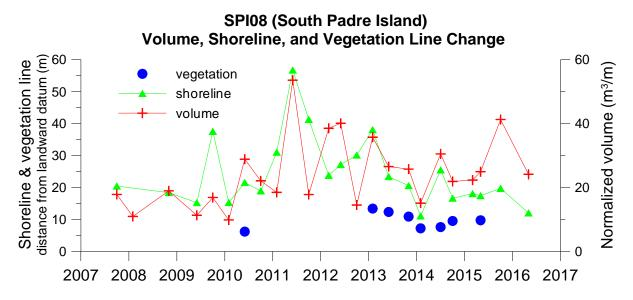
**Figure 18.** Volume and shoreline changes at SPI08 on South Padre Island due to beach-nourishment projects and the installation of sand fences.
