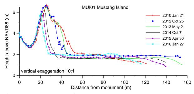
Figure 20. Excavated dune profile at MUI01 on Mustang Island.
