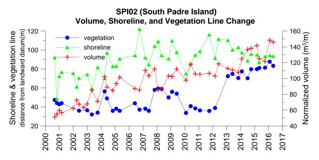
**Figure 17.** Changes at SPI02 on South Padre Island due to beach-nourishment projects and the installation of sand fences.
