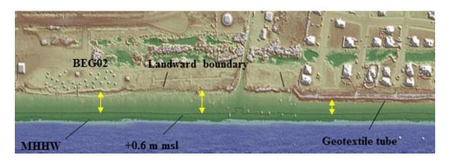
**Figure 10.** Lidar topographic-relief image of Galveston Island State Park and Pirates Beach subdivision. Note the difference in beach width between the natural beach and the area in front of the subdivision. From Gibeaut and others (2003).
