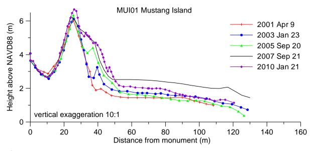
Figure 19. Foredune expansion at MUI01 on Mustang Island.
