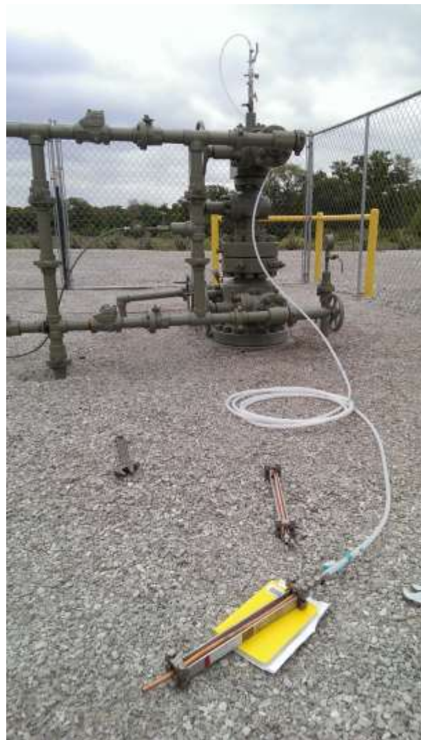
Figure 12. Produced gas sampling in the Barnett Shale area showing (a) IsoTube® for hydrocarbon and atmospheric gas collection and (b) copper tube for noble gas analysis.
