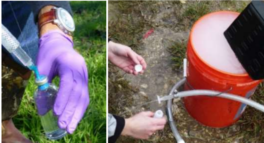
Figure 9. Dissolved gas sampling (a) and methane exsolving (Barnett Shale area)
