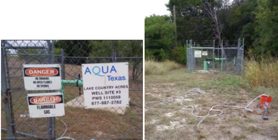
Figure 6. Water sampling for noble gas analysis (a) at the wellhead and (b) removed from the wellhead but before the tank (Barnett Shale area)
