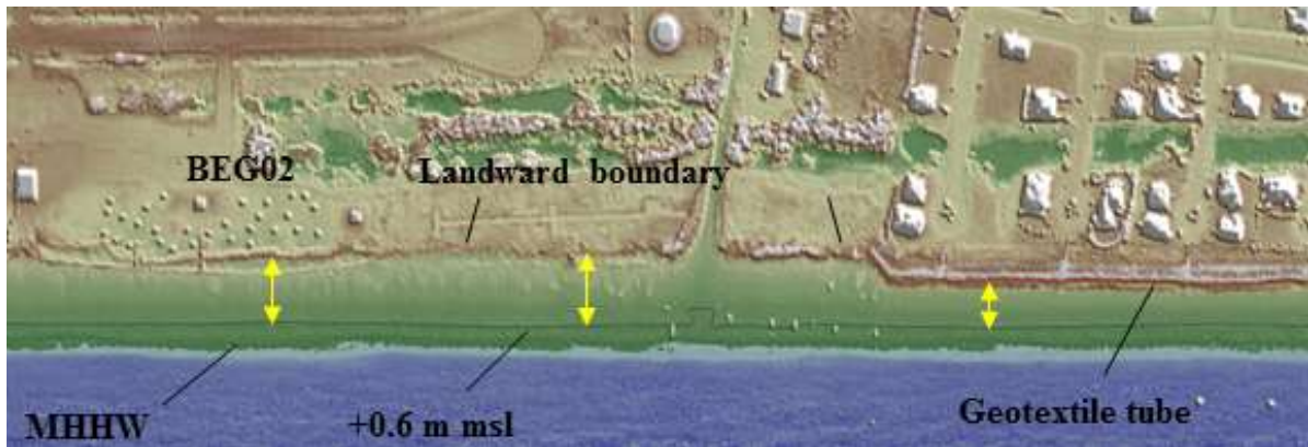
Figure 9. Lidar topographic-relief image of Galveston Island State Park and Pirates Beach subdivision. Note the difference in beach width between the natural beach and the area in front of the subdivision. From Gibeaut and others (2003).
