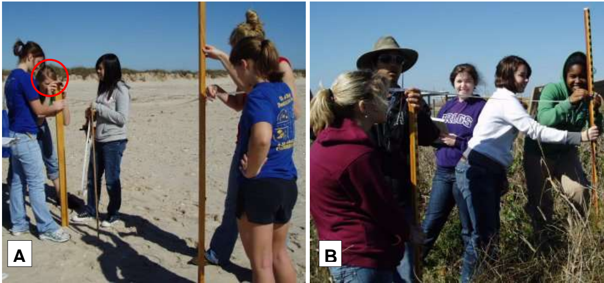
Figure 2. Students using (A) a sighting level to determine vertical offset between Emery rods, and (B) a metric tape to measure horizontal distance.
