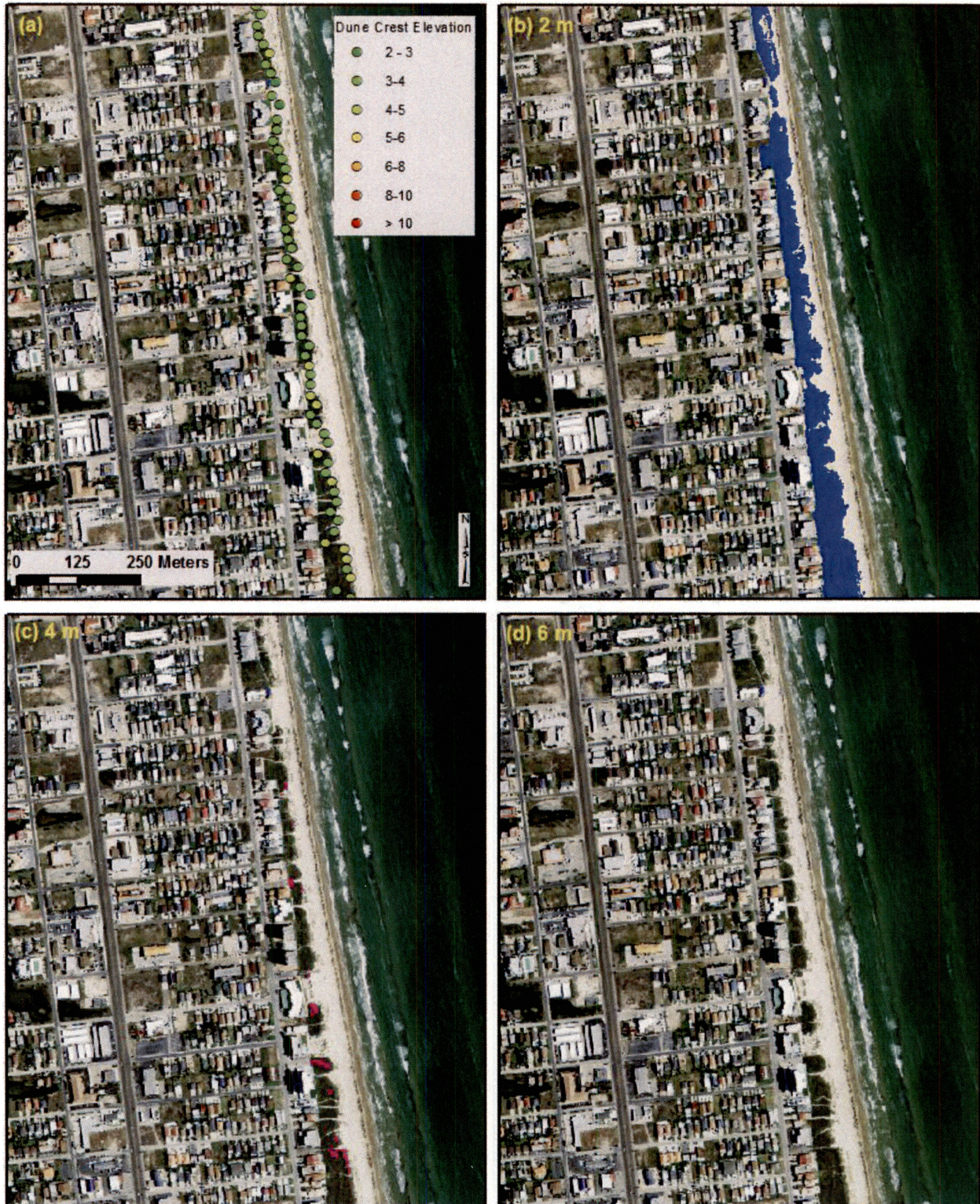
Figure 27. South Padre Island developed segment with seawall (a) showing maximum dune crest elevations. Areas of threshold elevations greater than (b) 2 m, (c) 4 m, and (d) 6m. Note there are no areas greater than 6 m in the beach and dune system.
