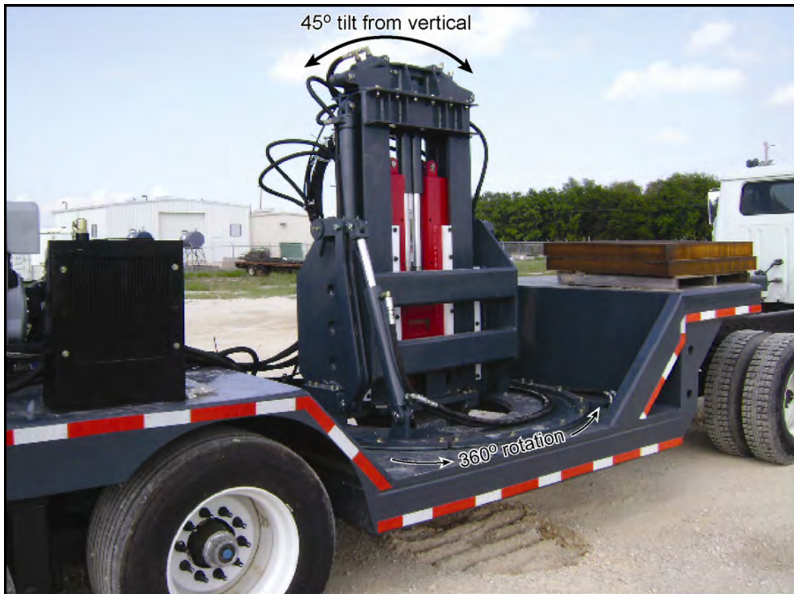
Figure A9. VSX™ accelerated-weight impact source provided by Vecta Technology and United Services Alliance. This source can deliver a vertical impact to the earth, or an inclined force vector can be applied in any azimuth direction and at any incident angle between 0 and 45 degrees without moving the vehicle. Vehicle weight is 33,000 lb. Its compressed-nitrogen spring system delivers 22,276 ft-lb (30,202 joules) of energy to the earth.
