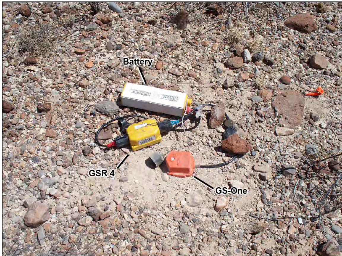
Figure 4.4. Photo showing the equipment deployed at each receiver station. Less than one meter of cable is required at each station, leading to the term “cable-free” to describe the technology utilized in this test. Equipment specifications are listed in Table 4.2.
