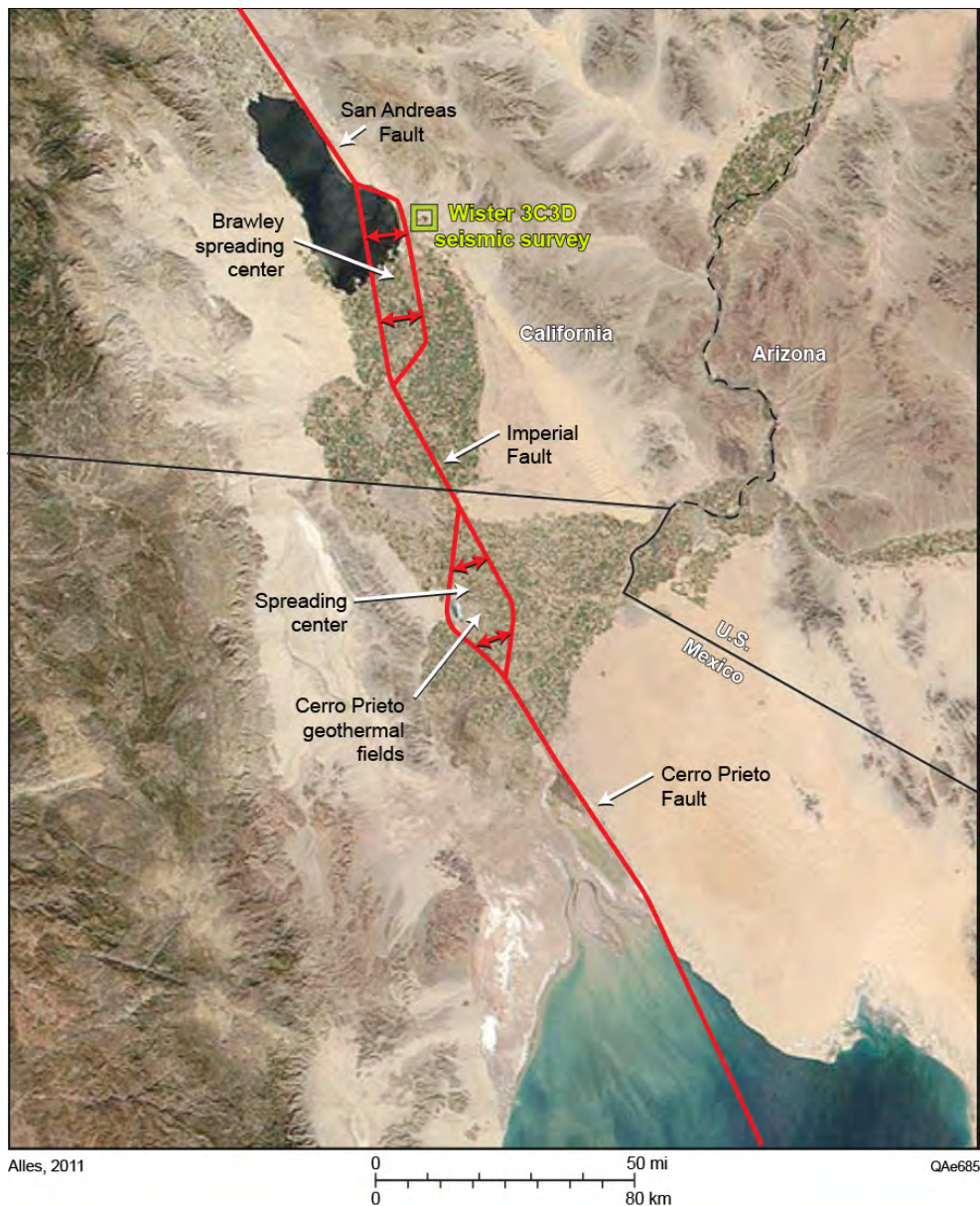
Figure 8.20. Location of Wister Field study area. Wister Field abuts the Brawley spreading center on the regional San Andreas fault. The largest geothermal field in Mexico, the Cerro Prieto Field, is approximately 100 km south on the same fault trend. Modified from Wallace (1990).
