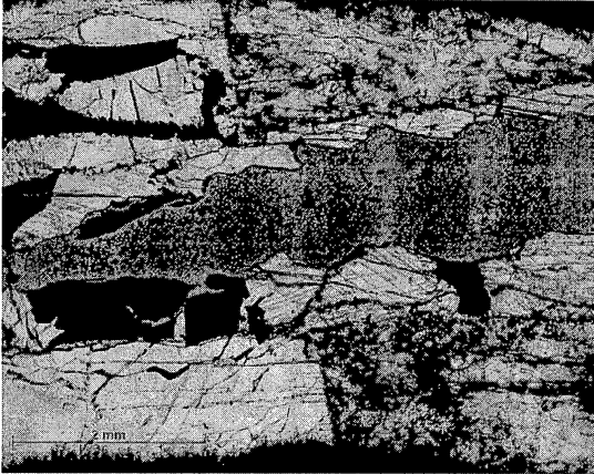
Figure 9. Fractured carbonate/pyrite concretions with multiple phases of fracture sealing cement, Hardie Unit #1 core. Samples from (a) 7,803 ft and (b) 7,817.5 ft. (c) Plane light photomicrograph of anhydrite, calcite and pyrite cements in the fracture in (a). These are similar to the fractures in the Paxton Isaac well concretions.
