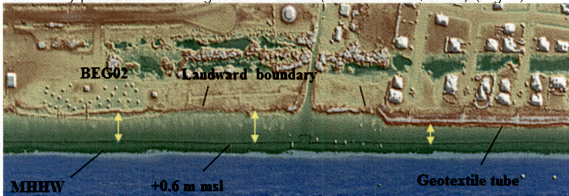
Figure 9. Lidar topographic-relief image of Galveston Island State Park and Pirates Beach subdivision. Note the difference in beach width between the natural beach and the area in front of the subdivision. From Gibeaut et al. (2003).
